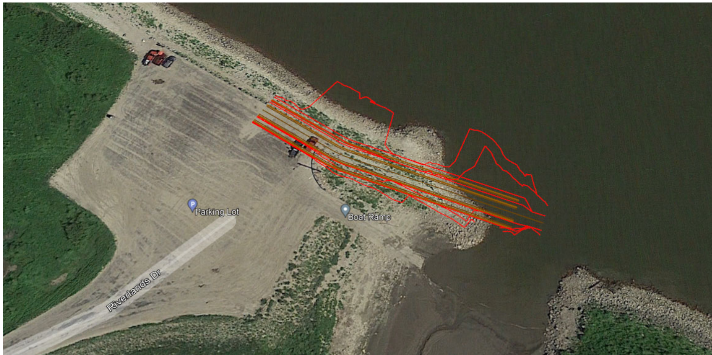
Figure 22. Proposed Boat Ramp Alignment
